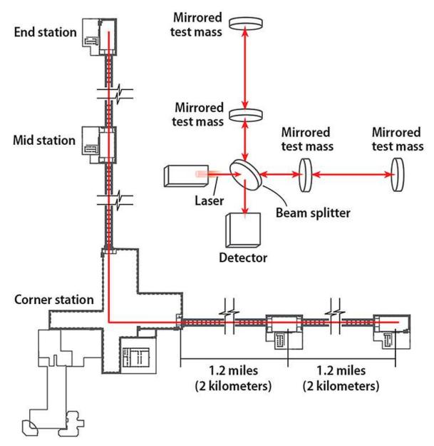
This diagram shows the layout of the observatory in Hanford, Washington. By making laser light travel up and down the arms and interfere with itself, scientists can deduce minute changes in the light's path from a gravitational wave encounter. *Astronomy*: Roen Kelly
