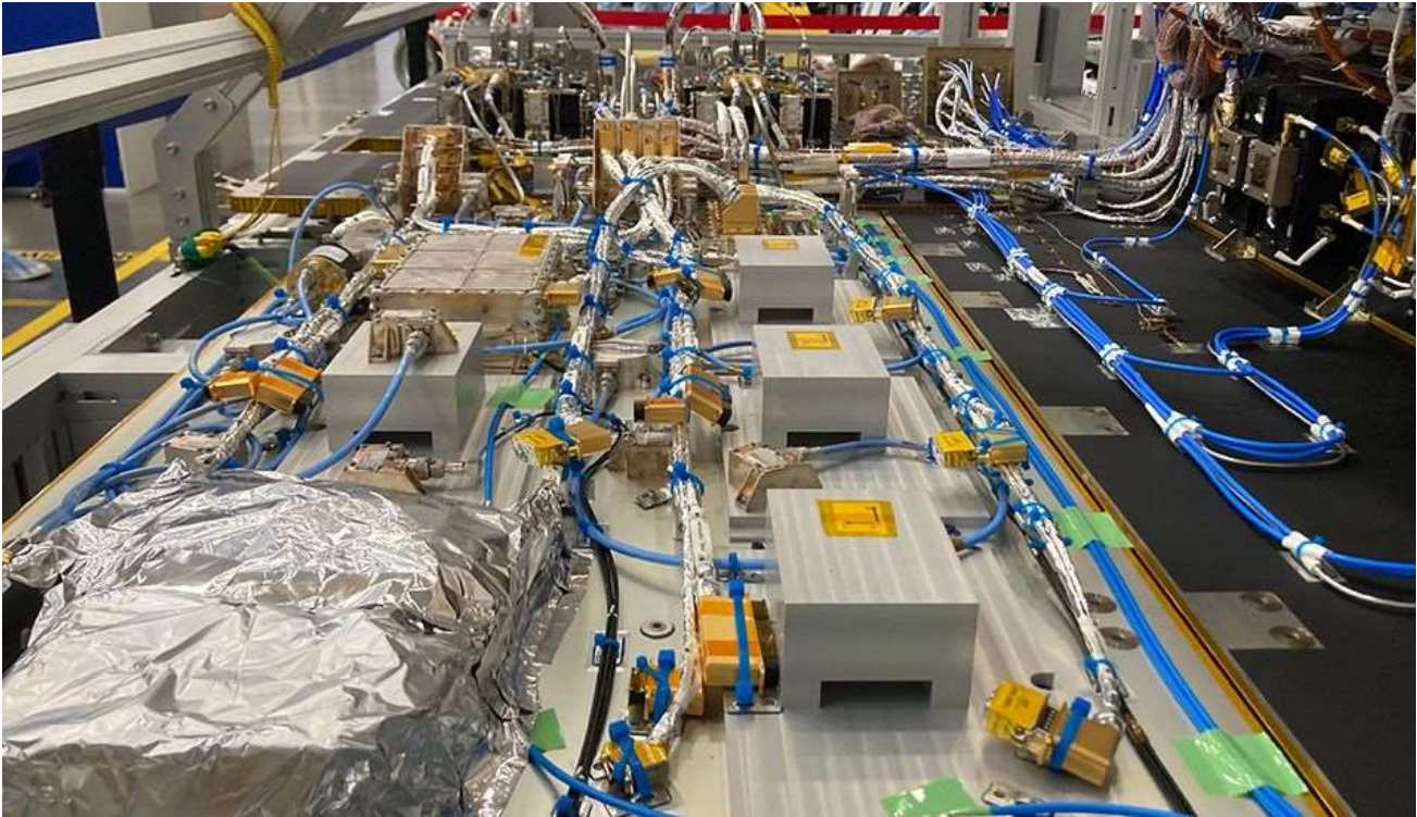
The radar electronics cover one wall of the satellite structure, or bus
