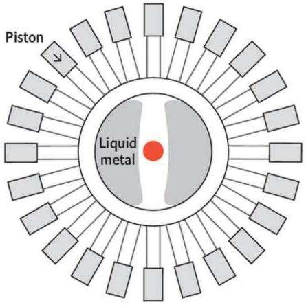
Plasma is compressed by the liquid metal lining of the reaction chamber, itself pushed inward by pistons
