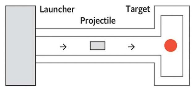
A projectile is accelerated down a tube. Hitting the target compresses a fuel capsule, triggering fusion
