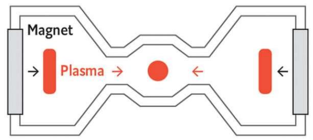
Plasma toroids at each end of the reaction chamber are propelled to the center, where they collide
